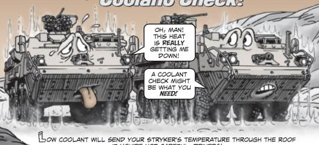
CHECKING COOLANT LEVELS AFTER EVERY OPERATION, JUST LIKE IT SAYS IN THE -10 TMS, WILL HELP YOUR STRYKER KEEP ITS COOL NO MATTER HOW HOT IT IS OUTSIDE.
